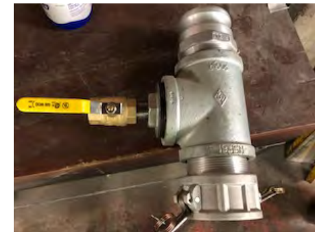
T-valve for pressure relief
